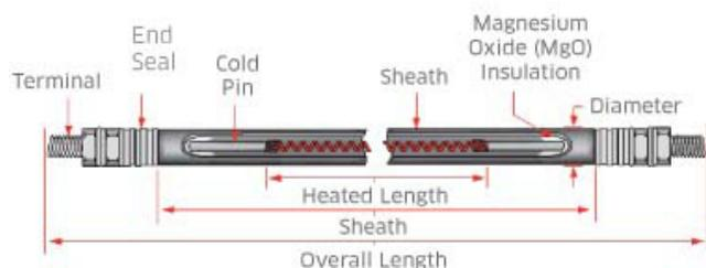
A tubular element has four basic components: a metal sheath, a helically wound coil of special resistive alloy, end seals, cold pins on each side of the coil, and magnesium oxide (MgO) insulating material. The tube is the outer casing of the heater and houses the other basic components. The cold pins protrude from the ends of the assembly to allow for power connections.
